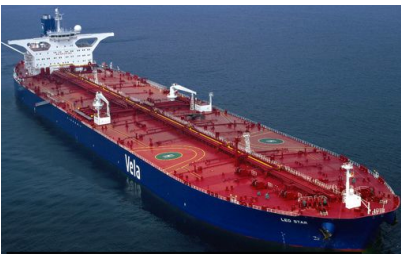
The Leo Star, a double-hulled supertanker capable of transporting 2 million barrels of crude oil, joins the Vela fleet (2002).
