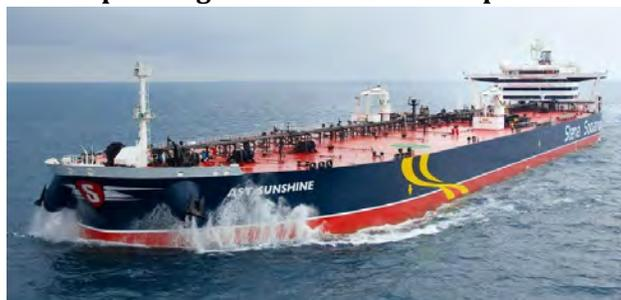
Suezmax tanker AST Sunshine, ordered and designed by Stena Bulk and Japanese Asahi Tankers, built at Samsung Heavy Industries, designed for energy efficiency, and launched in 2013. Flagged in Panama. Capacity is 159,000 DWT (1.16 Mb).
