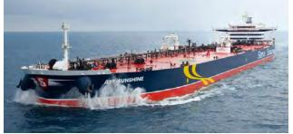
Suezmax tanker AST Sunshine, ordered and designed by Stena Bulk and Japanese Asahi Tankers, built at Samsung Heavy Industries, designed for energy efficiency, and launched in 2013. Flagged in Panama. Capacity is 159,000 DWT (1.16 Mb).
